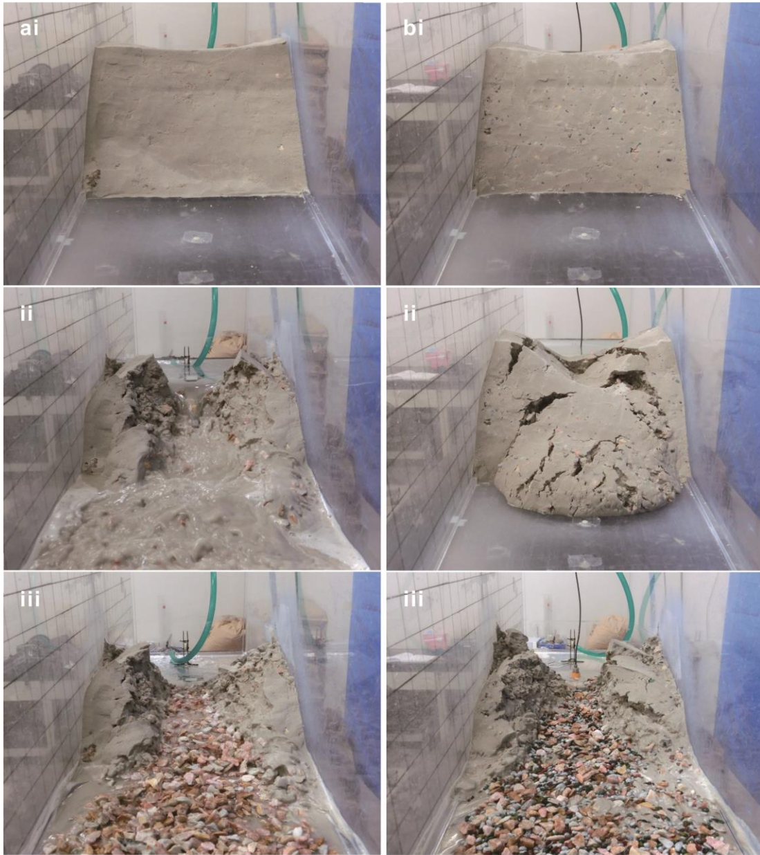
Figure 6.3 Photographic sequence of seepage-induced failure of dams built with (a) Gravelly dam I and (b) Gravelly dam II .
