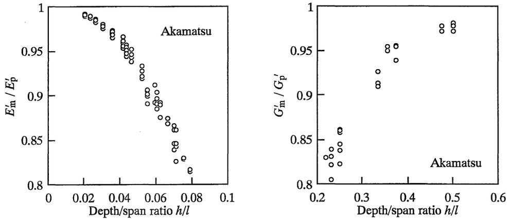
Fig. 4. Dependence of the values  $E'_m/E'_p$  and  $G'_m/G'_p$  on the depth/span ratio.
