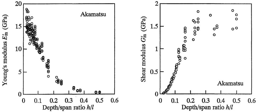
Fig. 3. Young's modulus  $E'_m$  and shear modulus  $G'_m$  calculated by neglecting the second and first terms in our proposal, respectively.
