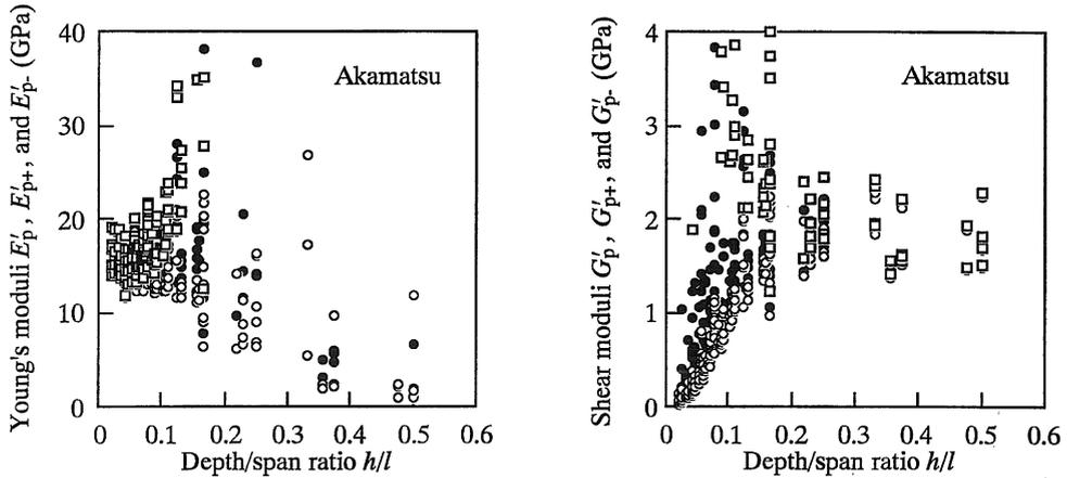
Fig. 2. Young's moduli  $E_p', E_{p+}'$ , and  $E_{p-}'$  obtained by substituting  $G_v, 1.3G_v$  and  $0.7G_v$ , respectively, and shear moduli  $G_p', G_{p+}'$ , and  $G_{p-}'$  obtained by substituting  $E_v, 1.3E_v$ , and  $0.7E_v$ , respectively, into modified equation.
