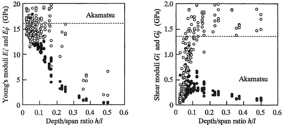
Fig. 1. Comparisons of the Young's moduli and the shear moduli obtained from original Timoshenko's theory and modified equation corresponding to the depth/span ratios.
