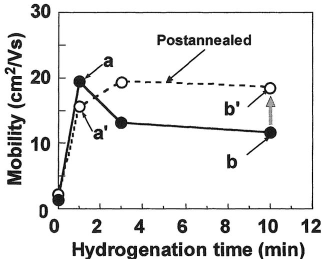
Fig. 3 Dependence of electron mobility on plasma-hydrogenation time, where poly-Si films were annealed at  $T_{pre}=600^\circ\text{C}$  to activate doped phosphorus prior to hydrogenation. The broken line shows mobility after post annealing at  $T_{post}=450^\circ\text{C}$  for 5 min. Raman spectra for samples labeled a, a', b and b' will be shown in Fig. 4.
