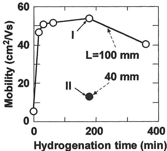
Fig. 7 Dependence of mobility on times of hydrogenation using hot-wire method. Distance between specimens and hot wire  $L$  is 100 mm (open circles) or 40 mm (closed circle).
