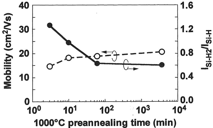
Fig. 12 Mobility and intensity ratio of Raman spectra for Si-H<sub>2</sub> to Si-H plotted as a function of time of preannealing at 1000°C. The samples were plasma-hydrogenated for 10 min after preannealing.
