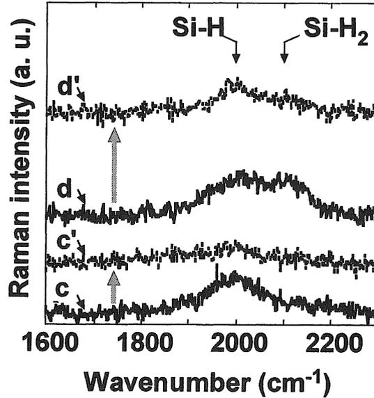
Fig. 11 Raman spectra related to Si-hydrogen bonds for samples plasma hydrogenated for 1 and 10 min after preannealing at  $T_{pre}=1000^{\circ}\text{C}$ . Labels c, c', d and d' correspond to those in Fig. 10.
