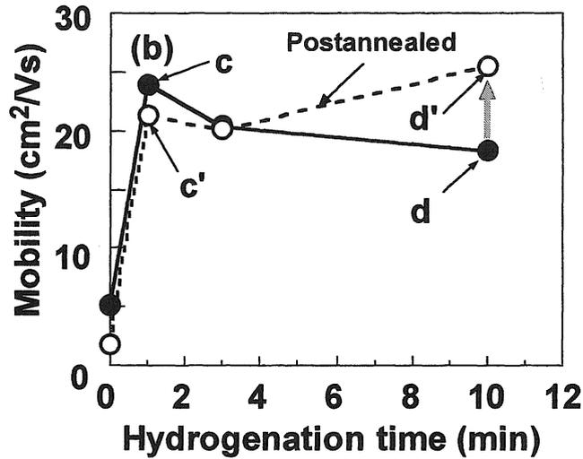
Fig. 10 Dependence of electron mobility on plasma hydrogenation time, where poly-Si films were preannealed at  $T_{pre}=1000^{\circ}\text{C}$  to eliminate in-grain defects. The broken line shows mobility after post annealing at  $T_{post}=450^{\circ}\text{C}$  for 5 min. Raman spectra for samples labeled c, c', d and d' will be shown in Fig. 11.
