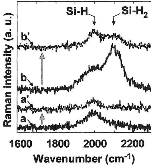
Fig. 4 Raman spectra related to Si-hydrogen bonding stretching modes of poly-Si films plasma hydrogenated for 1 and 10 min. Labels a, a', b and b' correspond to those in Fig. 2.
