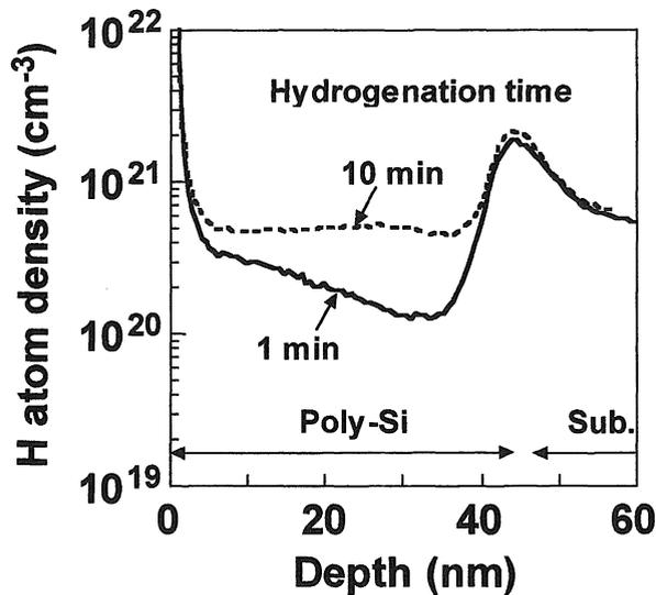
Fig. 5 Profiles of hydrogen-atom density in poly-Si films hydrogenated with plasma for 1 and 10 min. Measurement was made by using SIMS.
