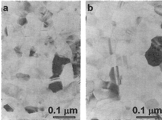
Fig. 9 Plan-view TEM images of poly-Si films annealed at (a)  $T_{pre}=600^{\circ}\text{C}$  for 2 min and (b)  $T_{pre}=1000^{\circ}\text{C}$  for 10 min. In-grain defects were eliminated at the higher temperature although grain size remained constant.
