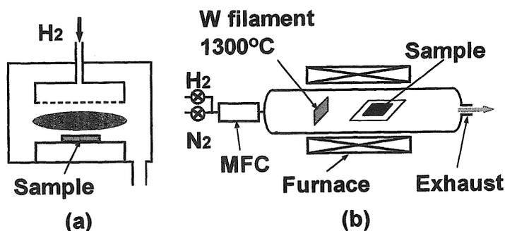
Fig. 2 Setup for hydrogenation of poly-Si. Atomic hydrogen was generated from  $\text{H}_2$  by using (a) the apparatus for PECVD and (b) a tungsten filament as the hot-wire catalyzer in a quartz tube evacuated to 0.1 Torr.
