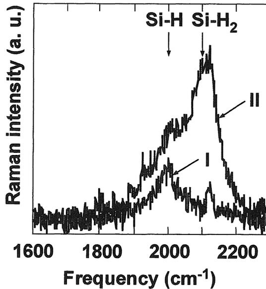
Fig. 8 Raman spectra after hydrogenation for 180 min by hot-wire method. Labels I and II correspond to those in Fig. 7.
