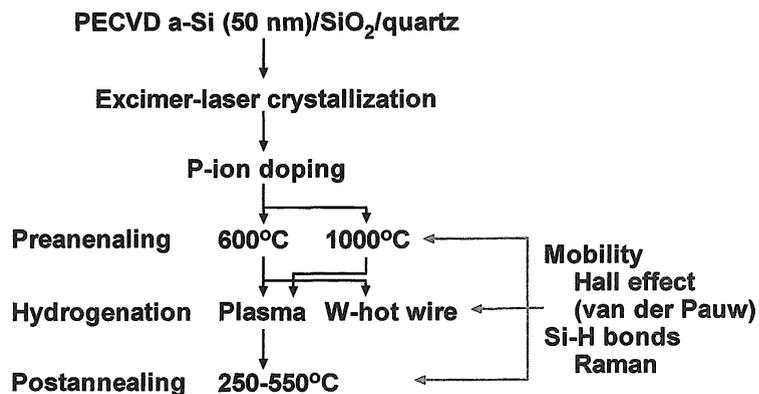
Fig. 1 Procedures of sample preparation and characterization.
