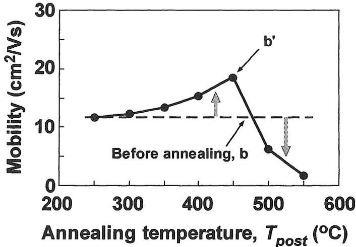
Fig. 6 Relationship between the mobility of excessively hydrogenated (10 min) samples and temperature of postannealing after this hydrogenation,  $T_{post}$ . The broken line demonstrates the mobility before postannealing. Labels b and b' correspond to those in Figs. 2 and 3.
