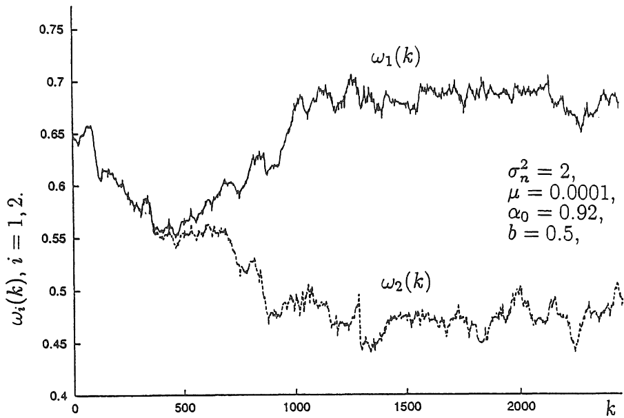
Fig. 7. The convergence behavior of \omega_i(k) , i = 1, 2 , for u(k) = e^{j0.7k} + e^{j0.5k} + \sqrt{0.5}(n_r(k) + jn_i(k))
