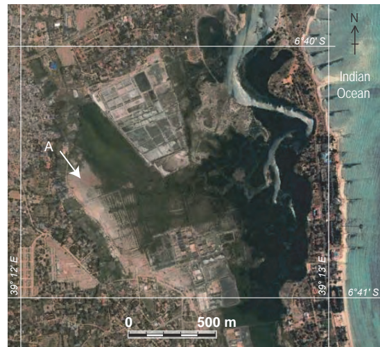
Fig. 5. Photo image showing construction of salt farm in mangrove area in Kunduchi (Fig.4). Square shapes are salt ponds for evaporation of sea water. Arrow indicates the land changed to red soil after deforestation of mangroves (see text).
