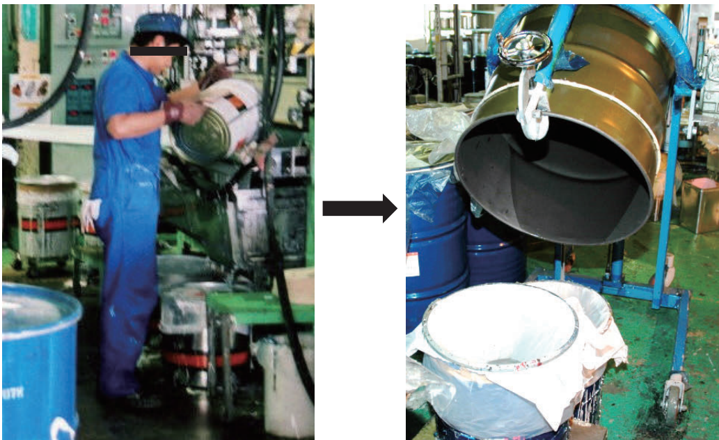
Fig.5. Instance of counter measures. (a) was an upgrades in efficiency local ventilation equipment; (b) was a mechanization of the ejection system of the coating solution
