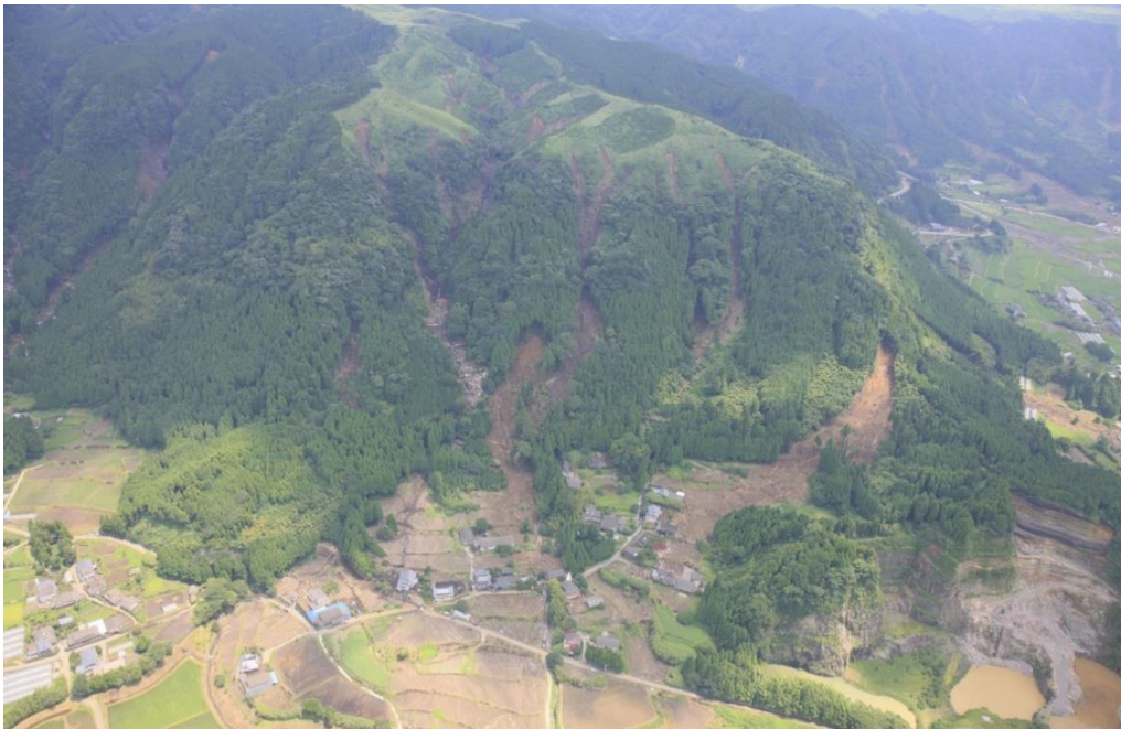
Fig. 4.1 Shallow landslides on the northeastern rim of Aso caldera (image courtesy of Kokusai Kogyo Co., Ltd, Japan)
