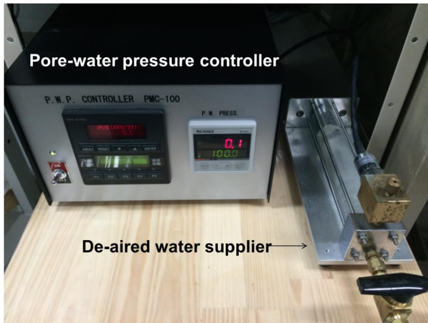
Fig. 3.4 Pore-water pressure controller system
