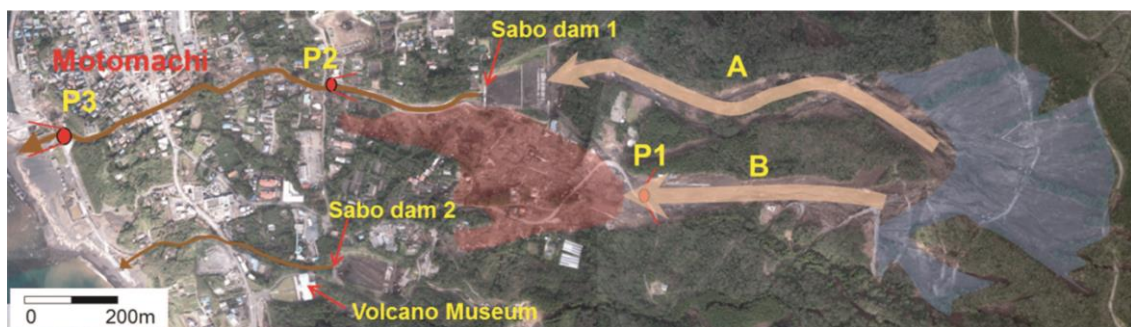
Fig. 5.7 Plan view of the main landslide area (photograph from the Geospatial Information Authority of Japan)
