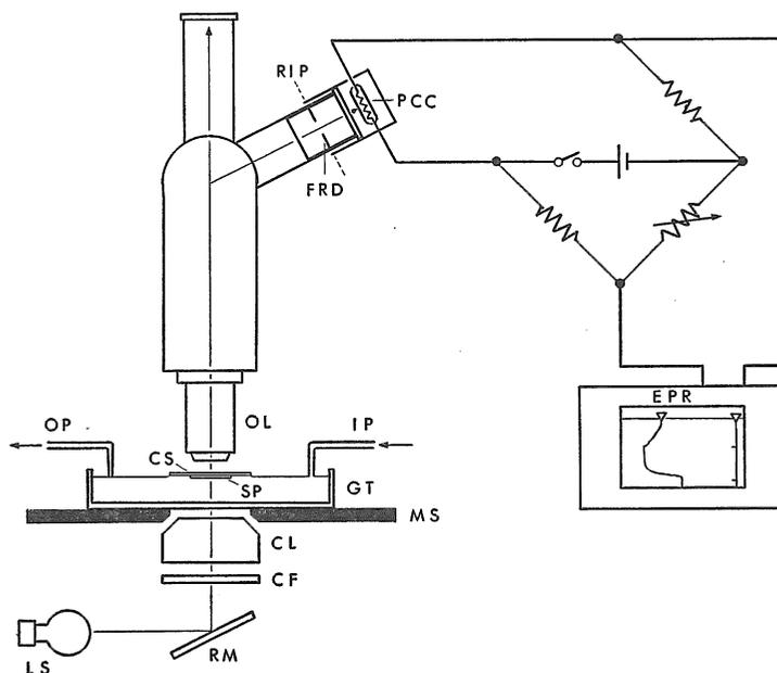
Fig. 1. A diagram of the experimental apparatus for recording melanophore responses *in vitro*.
