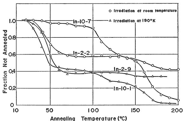
Fig. 2. Dependence of the annealing curves of indium-doped samples on the irradiation temperatures.
