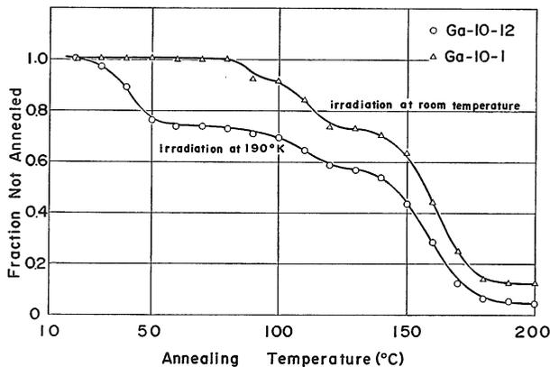
Fig. 1. Dependence of the annealing curves of gallium-doped samples on the irradiation temperatures.
