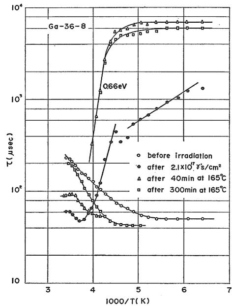
Fig. 7. The recombination behaviour of Ga-36 following irradiation by Co 60 gamma rays and successive annealings. A deep trap at  $E_c - 0.66$  eV is dominant after annealing.
