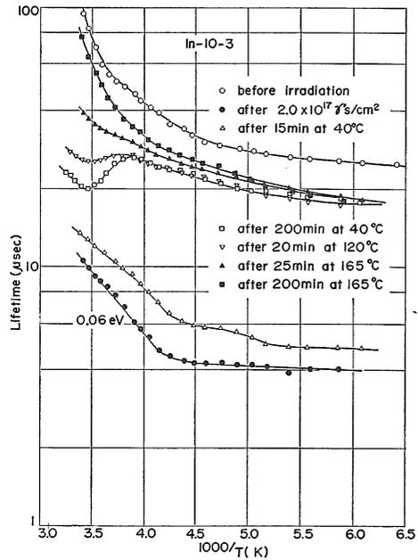
Fig. 5. The recombination behaviour of In-10 following irradiation by Co 60 gamma rays and successive annealings.
