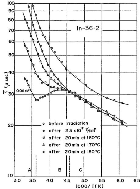
Fig. 3. The recombination behaviour of In-36 following irradiation by Co 60 gamma rays and successive annealings. A recombination level at  $E_v+0.06$  eV is dominant immediately after irradiation.
