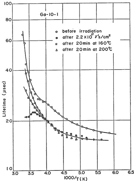
Fig. 8. The recombination behaviour of Ga-10 following irradiation by Co 60 gamma rays and successive annealings.
