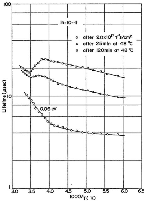
Fig. 6. The recombination behaviour of In-10 following irradiation by Co 60 gamma rays and successive annealings in the LT stage.
