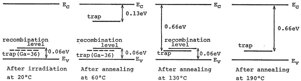
Fig. 10. Energy level scheme in irradiated *p*-type germanium.
