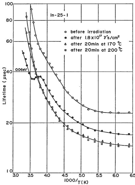
Fig. 4. The recombination behaviour of In-25 following irradiation by Co 60 gamma rays and successive annealings.
