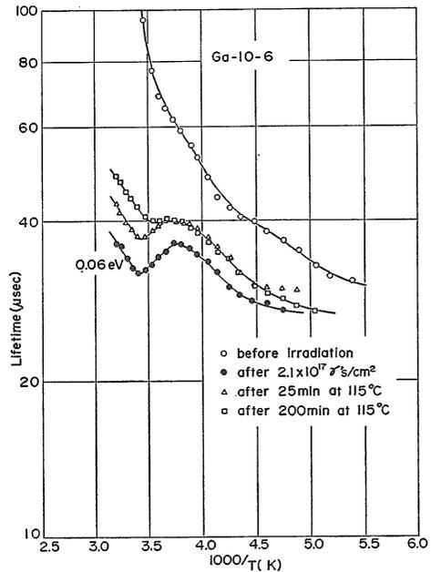
Fig. 9. The recombination behaviour of Ga-10 following irradiation by Co 60 gamma rays and successive annealings in the IT stage.
