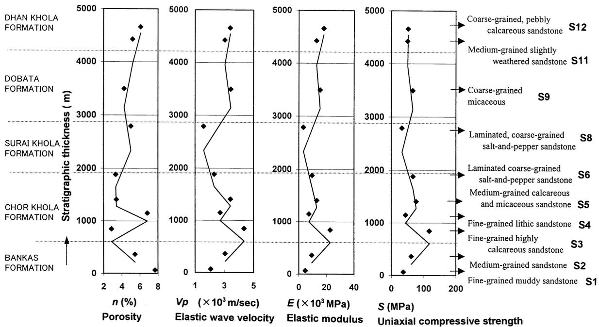
Fig.6 Stratigraphical changes of physical and mechanical properties of sandstones.
