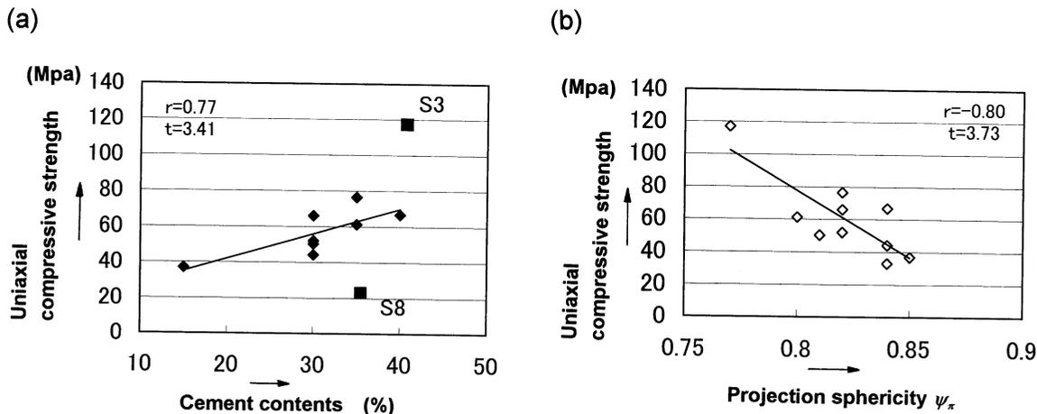
Fig.8 Relationship of uniaxial compressive strength with cement-content (a) and projection sphericity (b).
