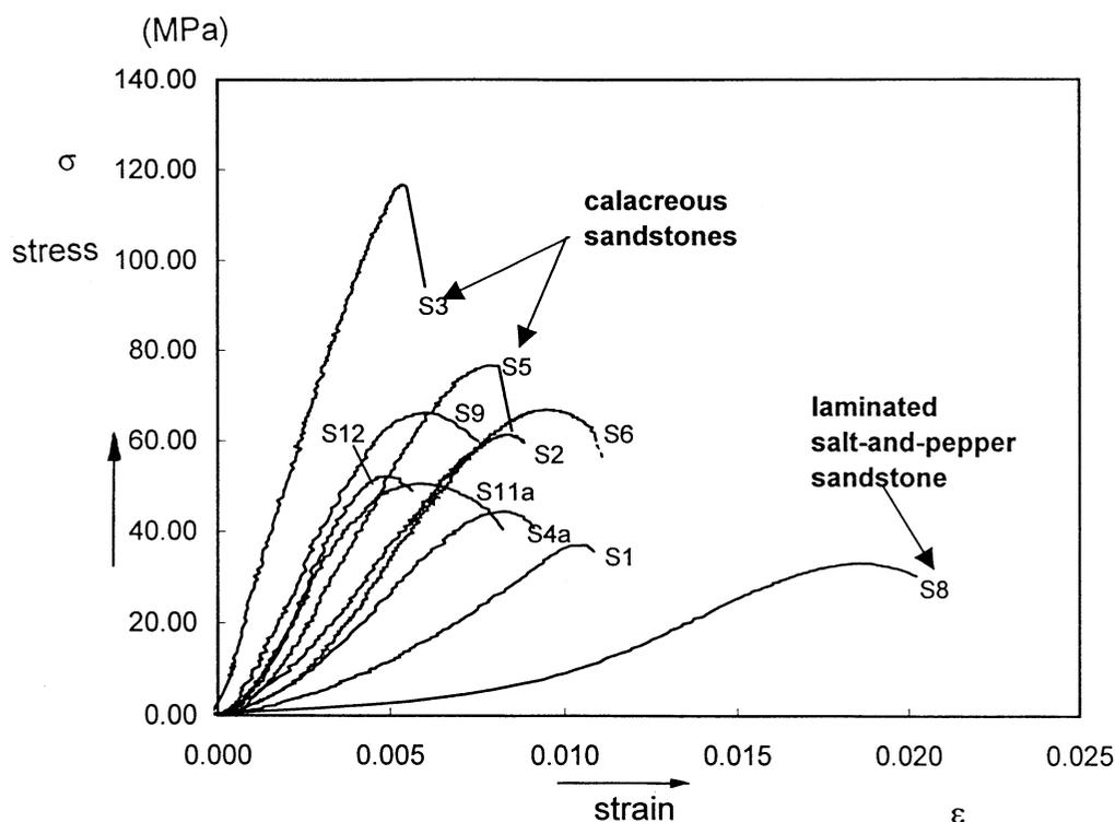
**Fig.5** Stress-strain relations in uniaxial compressive test of sandstones. Displacement rate of compression was set in 0.02 to 0.04mm/min.
