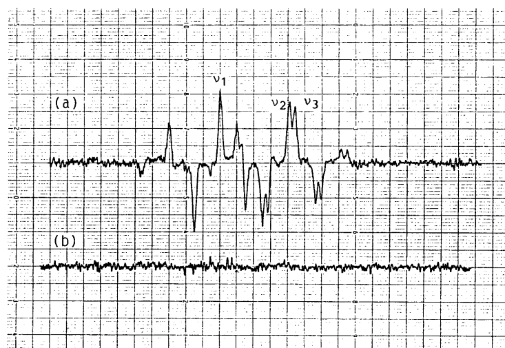
Fig.4. ^{35}\text{Cl} NQR spectrum for [\text{ICl}_2^+][\text{AlCl}_4^-] at room temperature (Zeeman field amplitude 10 mT; modulation frequency, 80 Hz; time constant, 5sec). (a) In-phase and (b) quadrature signals are shown. The resonance frequencies for the \nu_1 , \nu_2 , and \nu_3 lines are 11.423, 11.316, and 11.305 MHz, respectively.
