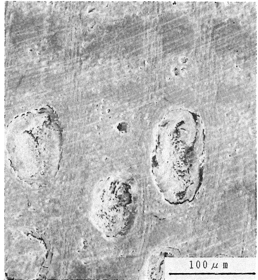
Fig. 9 Finish surface of cross section of keyaki in face turning.
