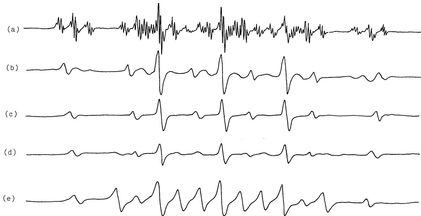
Fig. 3 ESR spectra of piperidinyl-1-oxy radical recorded at (a) -130^{\circ}\text{C} , (b) -90^{\circ}\text{C} , (c) -50^{\circ}\text{C} , (d) 0^{\circ}\text{C} , and (e) +110^{\circ}\text{C} .
