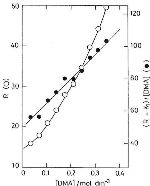
**Fig. 4.** R vs. [DMA] and  $(R - K_1)/[DMA]$  vs. [DMA] plots for the complexing of sodium ion in acetylacetone (DMA = dimethylacetamide)
