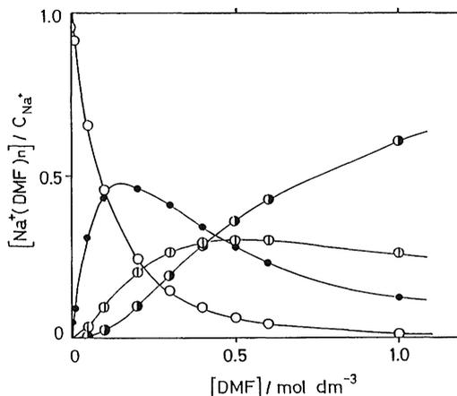
**Fig. 6.** Distribution of ionic species of sodium ion in acetylacetone + dimethylformamide (DMF) mixture ( $\circ$ );  $n=0$ , ( $\bullet$ );  $n=1$ , ( $\square$ );  $n=2$ , ( $\ominus$ );  $n=3$ ,  $C_{Na^+}$ ;  $0.001 \text{ mol dm}^{-3}$  (the total concentration of sodium ion)
