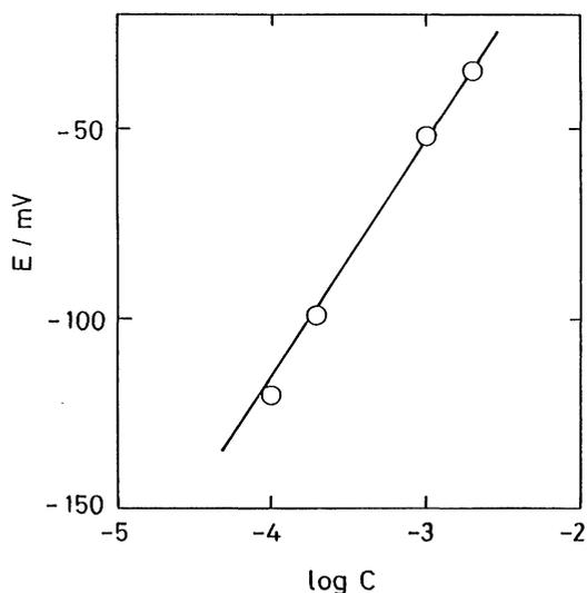
**Fig. 1** Relation between the potentials of silver wire electrode (E) and log C in acetylacetone
