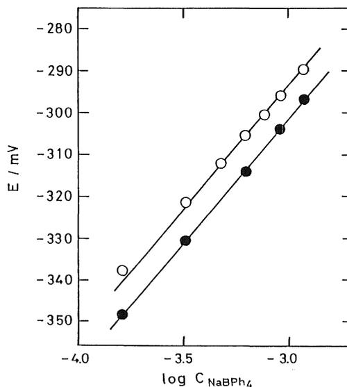
**Fig. 2** Relation between the potentials of sodium ion sensitive glass electrode (E) and log C in acetylacetone
