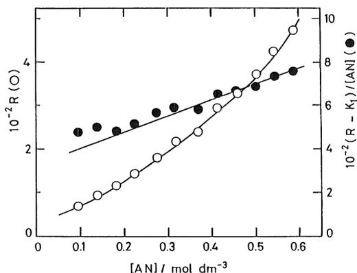
**Fig. 3.** R vs. [AN] and  $(R - K_1)/[AN]$  vs. [AN] plots for the complexing of silver ion in acetylacetone (AN = acetonitrile)
