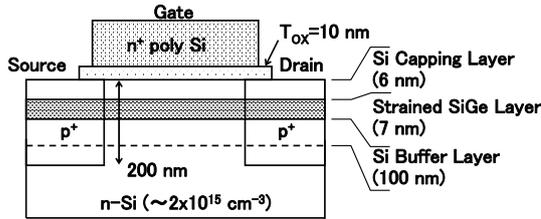
Fig. 1 Schematic cross section of SiGe-pMOSFETs
