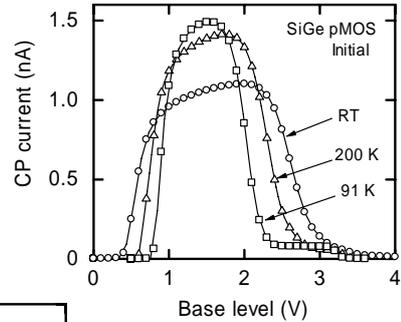
Fig. 2 Charge pumping characteristics before stress at RT and low temperatures.
