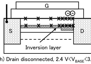
Fig. 4 Charge pumping characteristics measured under two different conditions, i.e., both source and drain terminals connected, and with the drain terminal disconnected, in a hot-carrier-stressed SiGe pMOSFET (a) at RT, and (e) at 91 K. Schematic representation of the inversion layer formed at the lower level of the gate pulse during charge pumping measurements in the indicated specific base level of the pulse, (b)-(d) at RT, and (f)-(h) at 91 K.
