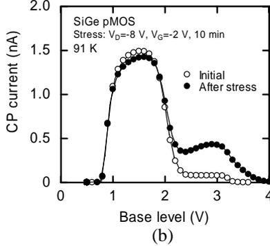
Fig. 3 Charge pumping characteristics before and after stress (a) at RT, and (b) at 91 K.
