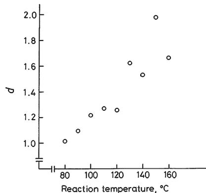
Fig. 4. Relative value of internal friction against reaction temperature due to the acylation by maleic anhydride for 2 h.
