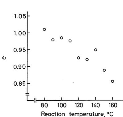
Fig. 3. Relative value of specific modulus against reaction temperature due to the acylation by maleic anhydride for 2 h.
