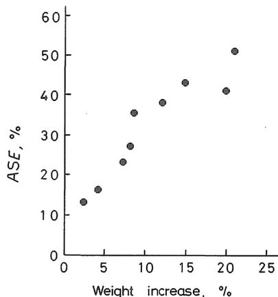
Fig. 2. Relationship between antismelling efficiency and weight increase due to the acylation by maleic anhydride.
