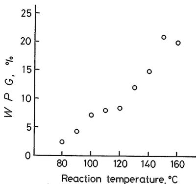
Fig. 1. Relationship between weight percent gain due to the acylation by maleic anhydride and reaction temperature for the reaction time of 2 h.
