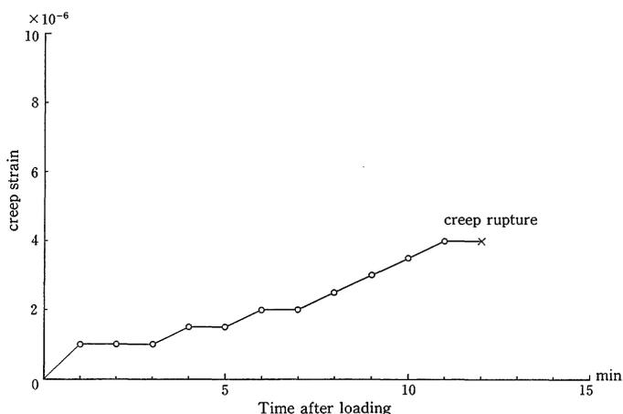
Fig. 9 Creep strain (Fly ash, loaded age 25, stress level 60%)
