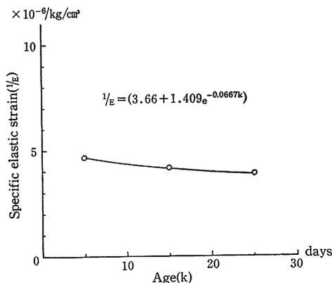
Fig. 5 Specific elastic strain-Testing age (Fly ash)
