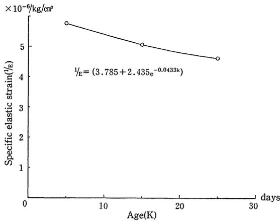
Fig. 3 Specific elastic strain-Testing age (Blast)
