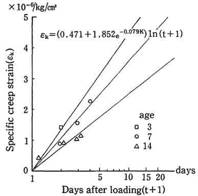
Fig. 2 Specific creep strain-Days after loading (Normal)
