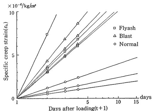
Fig. 8 Comparison of specific creep strain
