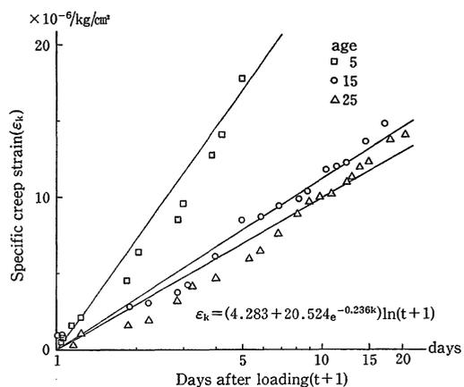
Fig. 6 Specific creep strain-Days after loading (Fly ash)
