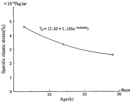
Fig. 1 Specific elastic strain-Testing age (Normal)
