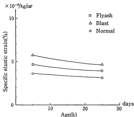
Fig. 7 Comparison of specific elastic strain
