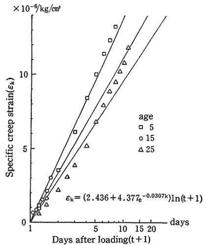
Fig. 4 Specific creep strain-Days after loading (Blast)
